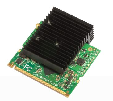
The new 2GHz super high power wireless card for long range links and powerful access points. This is the professional choice for reaching the last mile. 1.6W transmit power will give you the ability to reach even further than before. Up to 125Mbit throughput is possible with this device!
