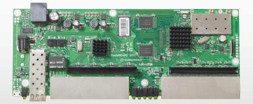
RouterBOARD 2011UAS-2HnD has most features and interfaces from all our Wireless routers. It's powered by the new Atheros 600MHz 74K MIPS network processor, has 128MB RAM, five Gigabit LAN ports, five Fast Ethernet LAN ports and SFP cage (SFP module not included!). Also, it features powerful (up to 1W!) dual chain 2.4Ghz 802.11bgn wireless, RJ45 serial port, microUSB port and RouterOS L5 license.
