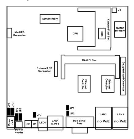
Note: on the other side of the board, there is only a MiniPCI connector, so no layout diagram shown.
